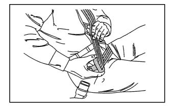
If the belt stops before it reaches the buckle, for lap-shoulder belts with cinching latch plates, tilt the latch plate and keep pulling the safety belt until it can be buckled.
